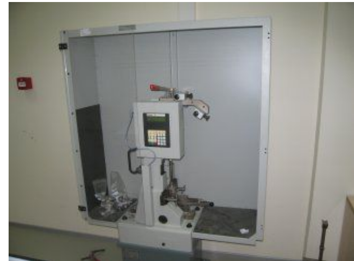
Charpy – Izod impact test system
