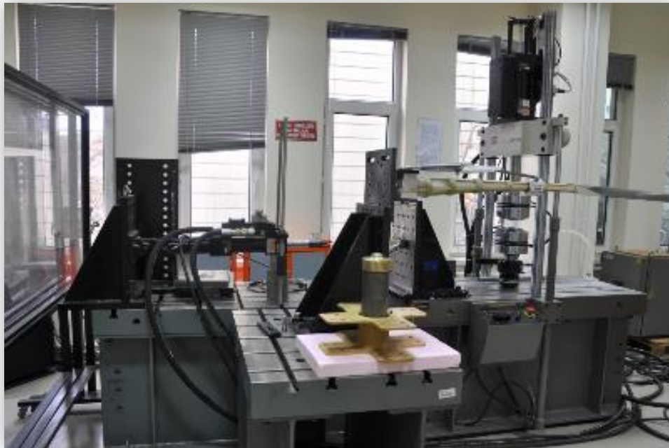
MTS testing frame: dynamical and statical testing
